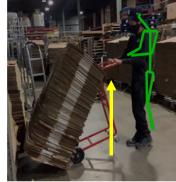
To remove product from the cart: lift the handle upwards keeping a neutral spine, then slowly tilt the trolley to place the stack on the ground.
